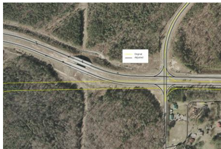
Street Centerline Misalignment and Adjustment
